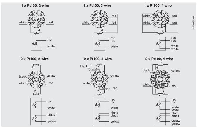
For the electrical connections of built-in temperature transmitters see the corresponding data sheets or operating instructions.
