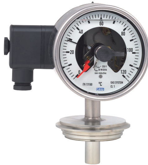
Gas-actuated thermometer with switch contact, model 74 with liquid damping and VARIVENT® connection
