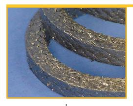
ML2001 is a pure homogenous graphite bonded to a fiberglass carrier for strength and thermal stability. It is Recommended for rotary and static applications associated with pumps and valves. ML2001 is available in bulk spools, spiral pack, and pre-cut or die formed ring sets. In addition, ML2001 will also be available with corrosion inhibitors for valve service.
