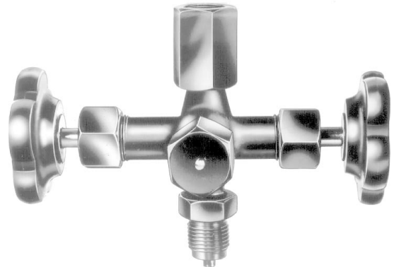
Valve with isolating test connection per DIN 16 272, LH/RH adjusting nut/Male G ½, with test connection M 20 x 1.5, PN 400
