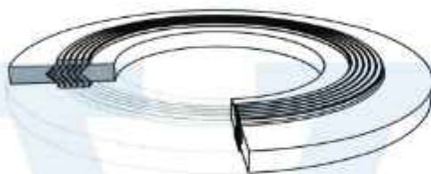
Form C/I, gasket with centering ring and inner ring
