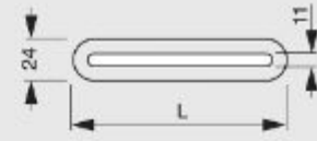
gasket graphite with SS-inlay for mica round, 24 mm wide
