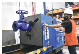
LEAKAGE AND PRESSURE TEST
